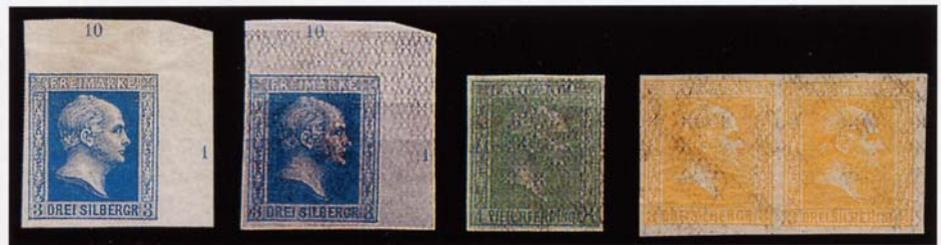
Typical lead sulfide damage of category III (far left: original condition)
