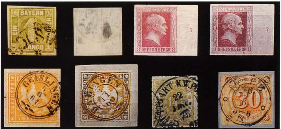
Further examples of typical lead sulfide damage (top row 3<sup>rd</sup> and bottom row 1<sup>st</sup> from left: original shades). According to our observations, some ten of thousands of partly valuable stamps have been damaged since 1975 due to being kept under PVC film.
