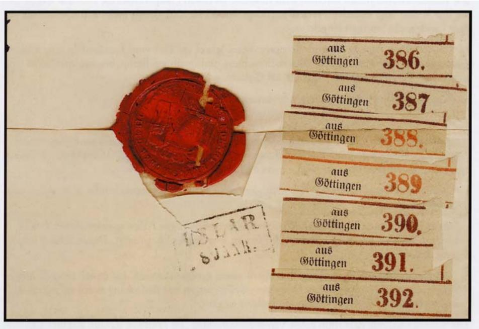
The more than 1mm thick wax seal created a cavity on this cover that had been kept under a PVC cover. The package labels attached in that area retained their original color. The others have become darker due to the direct contact with the PVC film.
